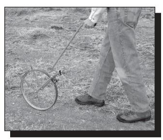
Figure 1—A measuring wheel can be used to measure the distance of the test course.
